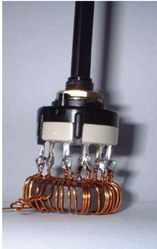
The toroid mounted on the coarse tuning switch. Note the radial taps in the bottom lefthand corner.
