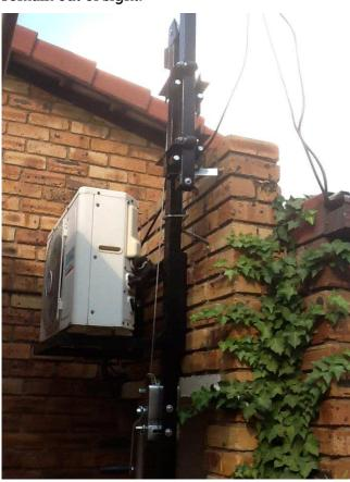
The antenna took a day or so to build and when installed at a height of roughly 4m above ground, was perfectly tuned for the lower portion of the 6m band(50.000-50.400).
