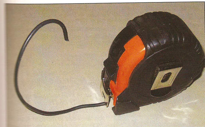
Figure 9 — Tape measure with soldered wire, fully retracted, ready for ring terminal.
