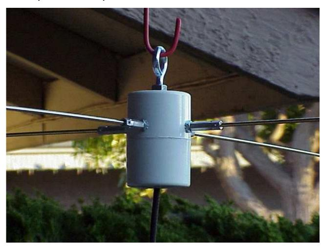
stores at higher cost, but you won't have to buy a pound of it for one antenna. The 1/8 diameter material is a slip-fit inside the 8-32 spacers. Cut the rods exactly in half, yielding two rods 18 inches long. This length plus the added length of the spacer and the case gives a good match in the 2-meter amateur band.
