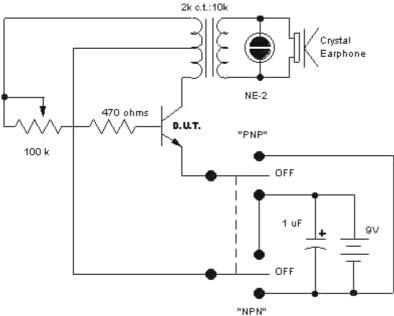
New transistor tester schematic
