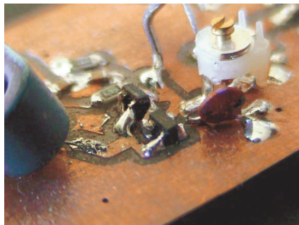
Fig. 6: push-pull configuration of two BF998. Input coil L1 is wound on 11 mm diameter core
