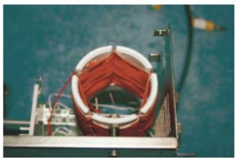
To combat this, I rewound the coil in a sort of "basket-weave" fashion. I cut slots into the coil form to create five plastic fingers. The coil wire was woven around these fingers, first over, then under, then over again. I eventually stopped when the coil reached 29 turns.
