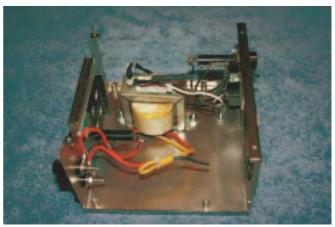
The "B" supply, like the Sanfordyne receiver itself, was built in a gutted PC power supply housing. The schematic can be viewed here.
