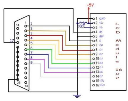
I came across this in my search for interesting articles for the Anode. The author [ ], has detailed several methods of "talking" to an Liquid Crystal Display (LCD) panel. All of which use the "common" HD4470 display driver chip.
