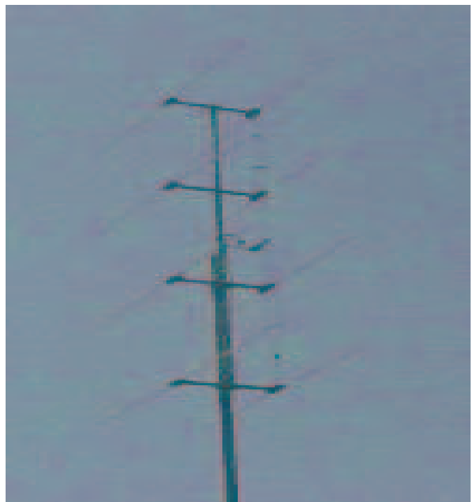
Figure 8. - four stacked half wave dipoles collinear antenna
