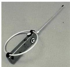
Adding a vertical "sense" whip or wire with proper signal phase resolves the rod or loop's inherent 180-degree ambiguity. More about the theory and practice of HF loops, rods and sense circuits is in the ARRL Handbook and my book "Transmitter Hunting----Radio Direction Finding Simplified."
