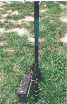
Long commercial fishing poles make excellent antenna supports for 80m ARDF transmitting. This one is at the 2003 USA ARDF Championships in Ohio. The transmitter and battery are in the weatherproof ammunition box.
