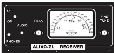
Fig. 4. Front panel decal. Actual size is 195mm by 90mm.
