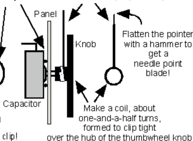
Flatten the pointer with a hammer to get a needle point blade!
