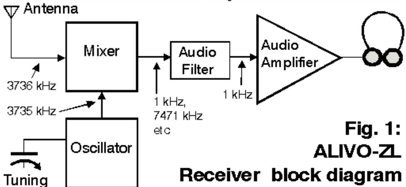
The output from the mixer is passed to an audio filter. The 1 kHz signal passes through and is amplified by the audio amplifier. The 1 kHz sound is heard in the phones. Changing the frequency of the oscillator with the tuning control - as the receiver is tuned across the band - will change the pitch of the audio signal you hear. SSB (single-sideband - speech) and CW (continuous wave - Morse code) signals can be 'tuned in' by careful adjustment of the tuning control.
