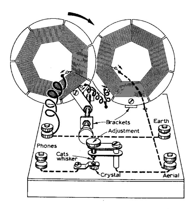
This drawing, showing the constructional details of the crystal set, should not be difficult to follow.
