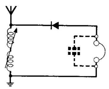
It could hardly be more simple! The suggested additional 'condenser' shown dotted can be about 1000pF. It will be cheaper to buy it rather than to follow the method described in the text for making a 'condenser'!
