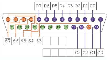
orientate aerial arrays, tune up **Printer Port Pin-out** valve finals and even print!
