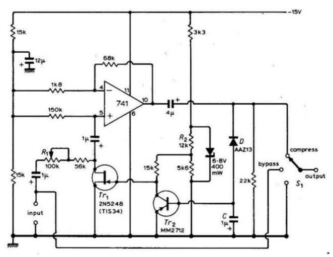
the a.g.c. mechanism appears as a modulation of the signal. It uses a readily available operational amplifier to provide a high input impedance and a well-defined gain. The low output impedance is used to drive the envelope detector D and its associated reservoir capacitor, Q thus giving fast reaction to spikes. The recovery time depends on C, (I have found 40-50 mS reasonable) and its minimum value must be com-
