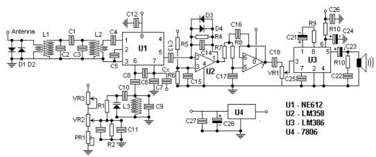
This is the circuit of the direct conversion receiver mentioned above. It is simple and easy to build. But requires an NE612 which is not so easy to source locally. The NE602 will not do as a substitute as the NE612 has an improved local oscillator circuit. JB
