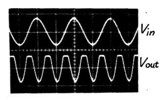
If the collector load resistor is replaced by a tuned circuit of only moderate Q-value, say. 10, a clean double-frequency sinewave output may be obtained.
