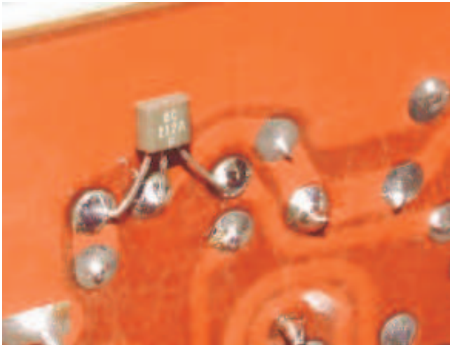
Transistor soldered to the under side of PCB BC212 replacing OC171
