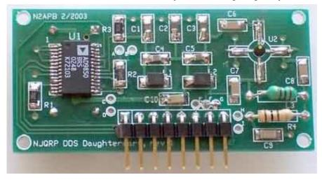
Build this simple, small AD9850-based DDS board and plug it into your favourite project to serve as a precise and stable signal source from the sub-Hertz basement all the way up to 30 MHz.
