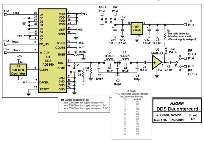
The controller's software just needs to send a 40-bit serial data stream on the DATA line with each bit being clocked by the CLK control line. At the end of the sequence, the LOAD line is toggled to instruct the DDS chip to use the new frequency—then bingo, the new frequency
