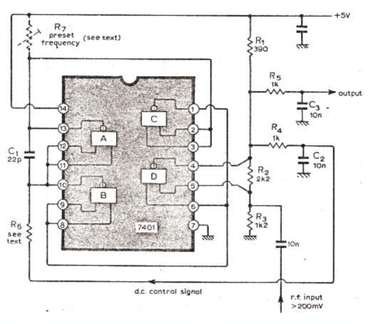
loop. A separate filter R5 and C3 provides the audio output.
