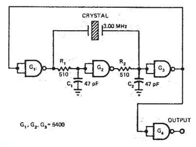
This loop-within-a-loop oscillator design requires no tedious selection of components to ensure reliable starting.
