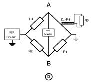
Fig a, when R1= R2 and, R3=R4, then the bridge is in balance and no current will flow through the centre arms. The R1, R2 combinations do not have be
