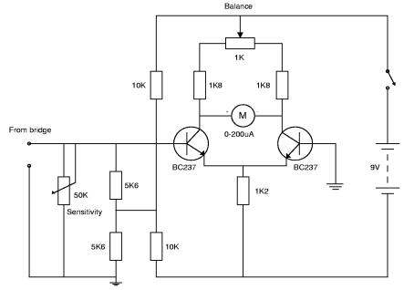
Fig - 3 Meter amplifier for the antennascope when a low power signal source is used. Meter is balanced for zero by
