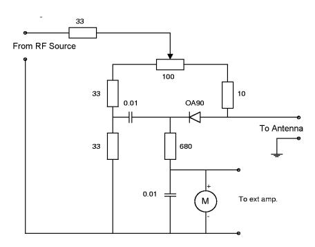
detector. As one arm of the bridge, (or the ratio of the two arms). changes from the balanced value, the bridge becomes unbalanced and the voltage detected across points A-B increases in proportion to the unbalance.
