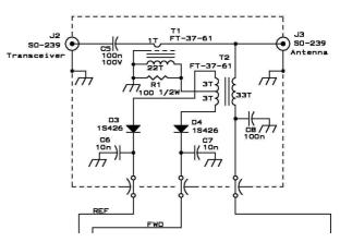
The sensing circuit he used (above) "broadband" and is one to emulate.
