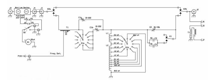
Instead of using a roller inductor, he used a switched inductor for the ATU. This seems to be a common choice of the AAT's makers. The rotary switch in many of the designs is replaced with a series of relays. The relays are again controlled by a small micro.
