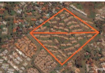
When reading about BPL, John was inspired by to try 'Reverse BPL' for his antenna system. Fortunately his QTH is placed roughly central in the complex. He built a Rhombic using the mains wiring of the complex. He savs. "Why not? We used the fence surrounding the RAF camp for an aerial long ago."
