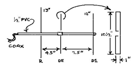
for SWR) and the director, but fessional just try taping the reflector to the boom first. After adjusting the driven element for best I used RG-8X and not the SWR at 436.8 MHz, you can more common RG-58. For an move the reflector slightly to equivalent 10' (2.5 m) of coax, get the SWR perfect. I used RG-58 has 1.2 dB loss while glue to hold the reflector and RG-8X has only 0.8 dB loss.
